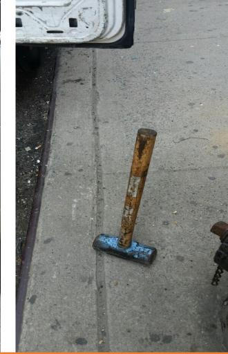
**PREVENTION: Material fall protection should be in** place ensuring tools are tethered.
