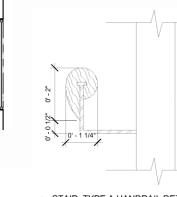
9 STAIR TYPE A HANDRAIL DETAIL 6" = 1'-0"
