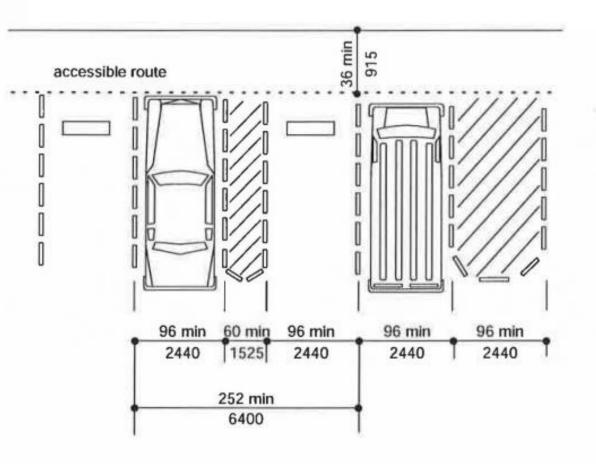
FIGURE C502.4.1(a) ACCESS AISLE CONNECTED TO AN ACCESSIBLE ROUTE
