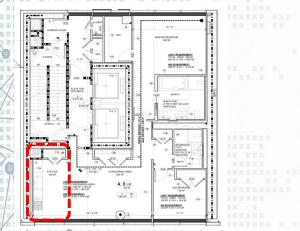
as per FHA Design Manua € of refrigerator Requirement 7. & CFS Part A, Page 7.6 depth of the Ref required air space the Ref OR REF 30" è 30"x48" forward approad 30"x48" CFS for Forward or Parallel Approach to Ref, As per 1. <u>FHA</u> Requirement 7(1)(a) 2. UFAS-Sec. 4.34.6.2
