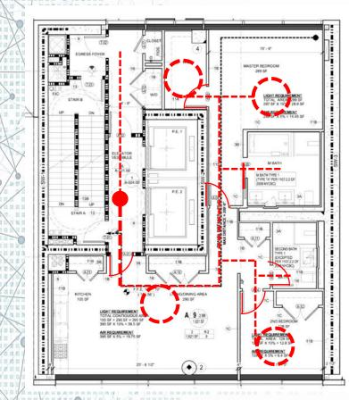
Primary Entrance – must be on an accessible route connecting with the accessible entrance(s) and common areas Accessible Route – all unit spaces and elements must be connected by an accessible route Walking Surfaces – accessible route walking surfaces must comply w/Section 403
