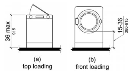
Figure 611.4 Height of Laundry Compartment Opening
