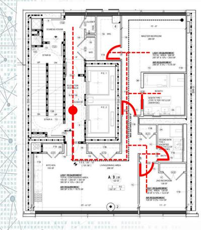
Primary Entrance – must be on an accessible route connecting with the accessible entrance(s) and common areas
