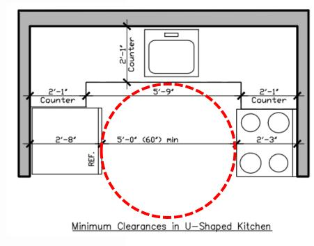
NOTE: Consider the most protruding element in the kitchen while calculating the clearances
