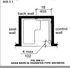
**608.2.3.2 Seat.** A folding seat complying with Section 610 shall be provided on the seat wall opposite the back wall.
