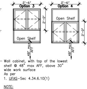
30" wide, taller wall cabinet above 30" wide work surface will provide reasonable storage space at an accessible height.
