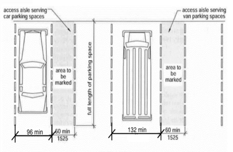
FIGURE 502.4 PARKING SPACE ACCESS AISLE
