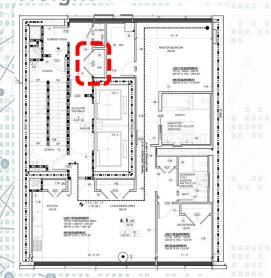
611.2 Clear Floor Space. A clear floor space complying with Section 305, positioned for parallel approach, shall be provided. For top loading machines, the clear floor space shall be centered on the appliance. For front loading machines, the centerline of the clear floor space shall be offset 24 inches (610 mm) maximum from the centerline of the door opening.
